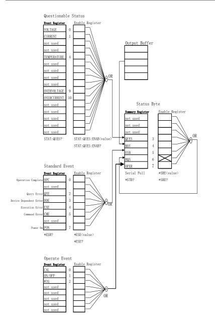
Event register is read only register, used to store the implementation status of the power, the data used in the event register latches in the form, once the data is stored, subsequent data will be completely ignored. Even can't changed by re-setting order (\* RST) or equipment restart.
